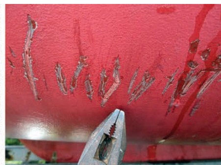
Beast from the east is small beer to a tough Kinsman. Just small scrapes through the GRP coatings, March 2018
