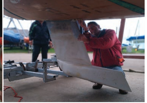
Exposed keel was cleaned, epoxied and reinstalled
