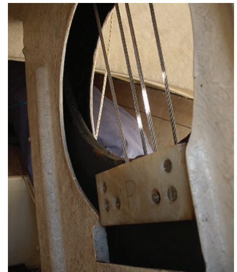
Top of keel in its keel box
