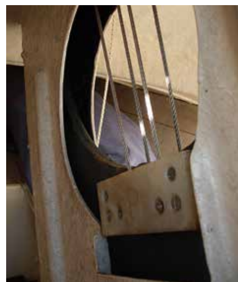
Top of keel in its keel box
